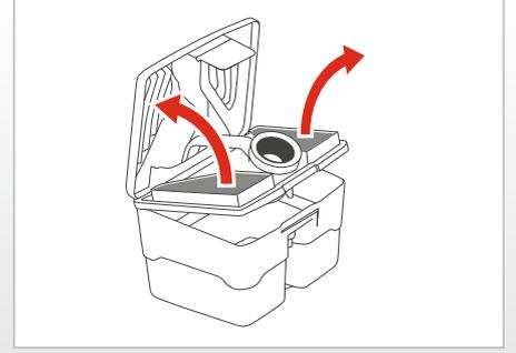
Exchanging the EPA filter and EPA prefilter
